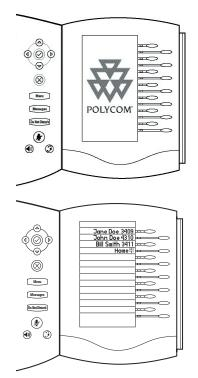
Power is automatically transferred from the host SoundPoint® IP 601 phone to Expansion Module(s) upon connection. Units may be plugged and unplugged (hotswapped) at any time to a live SoundPoint® IP 601 host phone.
