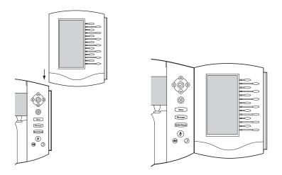
(3) To connect up to three Expansion Modules together, repeat steps ① and ②.
