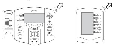
Align the Expansion Module at the top of the groove lines on the SoundPoint® IP 601 phone and slide unit downwards until unit clicks into position. Connect the Base Stand for each Module.
