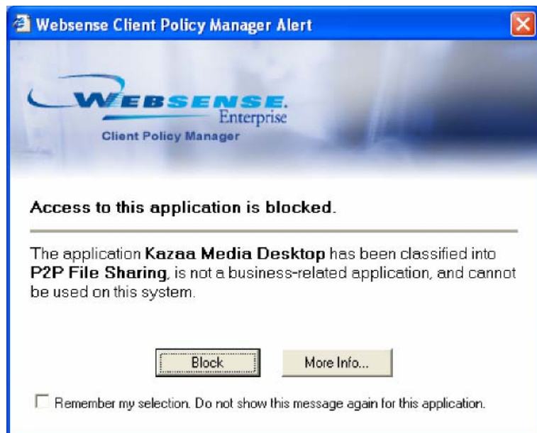
Figure 4 CPM blocks the launch of P2P applications on all employee computers, even when they are not connected to the network.
